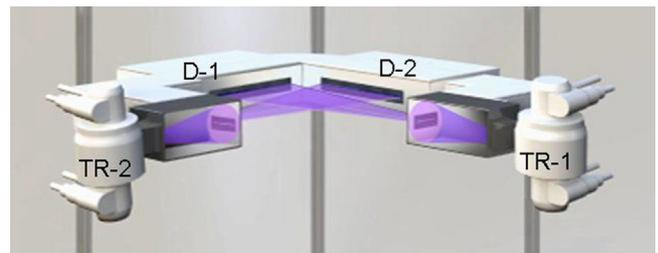
Fig. 2. Orthogonally co-linked X-ray tube (TR1 and 2)/detector (D1 and 2) pairs.
