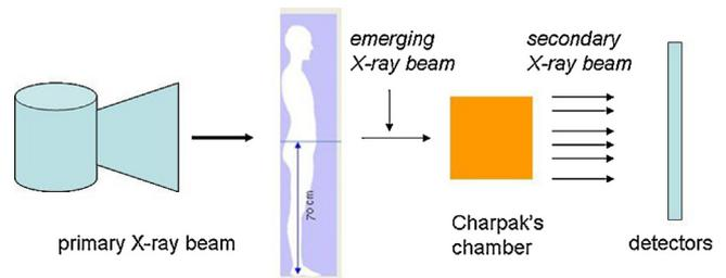
Fig. 1. Diagrammatic representation of the amplification of the low dose primary X-ray beam through the Charpak's chamber.
